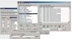
The Plena Replay Software runs on a PC and manages and replays playlists of BGM (stored in compact MP3 format). It also manages and replays digitally recorded messages at pre-programmed times. The software can be used with all Plena equipment.
