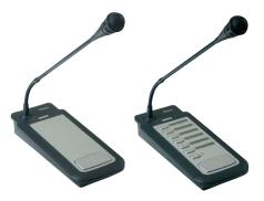
Plena Call Stations feature a flexible-stem condenser microphone with a stable metal base that also allows desk-top flush-mounting. There are all-call and 6-zone versions for use with the Plena System Pre-Amplifier. Selected zones and the active state of the microphone and system are indicated by LEDs on the call station. The call stations have selectable gain, a speech filter and limiter to improve intelligibility. Switches in the call station allow chimes to be selected.
