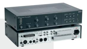
The Plena Multi-Zone Call System provides dual-channel operation (calls and BGM) for 6 zones. The unit is used with Plena Booster Amplifiers. It has two call station inputs, each to connect multiple cascaded call stations, a selectable filter for optimizing speech intelligibility, and separate volume control and tone controls for the speech and BGM channels. Six levels of priority are available for music, microphone, call stations, trigger inputs and the emergency input.
