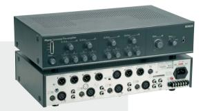
The universal pre-amplifier extends the configuration possibilities of the Plena family. It offers a choice of mixing, blocking or serial input priority modes. Each input channel has its own volume and tone controls, a selectable filter to optimize speech intelligibility, and direct outputs. On the output, it's also possible to override local loudspeaker volume controls to ensure an important message gets through.
