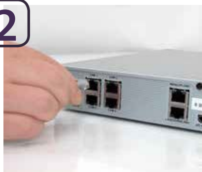
...to an appropriate port in the network video recorder...
